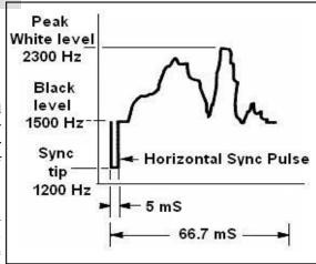
SSTV is not a digital mode like RTTY and PSK31. It is an analogue mode like SSB. It uses frequency modulation, whereby every different value of brightness of a spot in the image is represented by a different audio frequency. Color is achieved by sending the brightness of each color component (usually red, green and blue) separately and sequentially. On HF this audio signal is then fed into an SSB transmitter.
