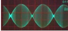
When running 100W PEP, the power meter of the transmitter will indicate 50 W, provided the transmitter is not overmodulated. A 100 W transmitter can be run at 100 W PEP (not average!) for long periods of time (the wattmeter indicating 50 W). The duty cycle is 50%.
